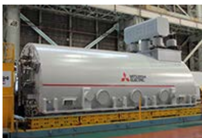
870 MVA generator for verification test
