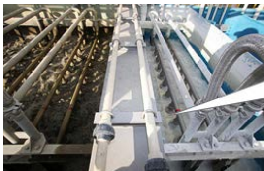
Water detoxification equipment at metal plating facility. Vat at left is for heavy metals; vat at right holds water containing fluorine.
