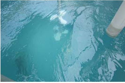
Water detoxified by microfiltration. It is further filtered by reverse osmosis (RO), which eliminates impurities like soluble salt. The water is used again for washing at the metal plating factory.
