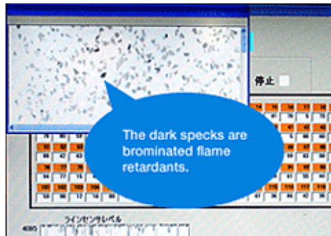
Award-winning technology where X-rays detect plastic chips containing flame retardant, and instantly instruct 124 individual air jets to blow them aside
