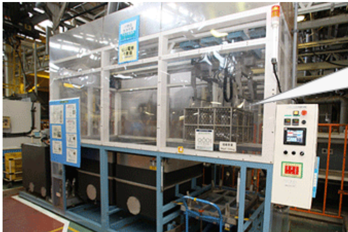
Microbubble cleaning equipment
