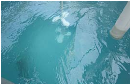
Water detoxified by microfiltration. It is further filtered by reverse osmosis (RO), which eliminates impurities like soluble salt. The water is used again for washing at the metal plating factory.
