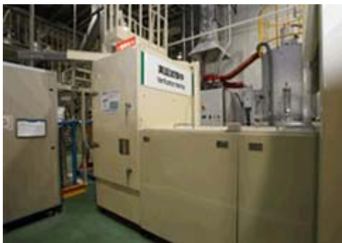
X-ray analysis separation equipment for eliminating plastic containing bromine
