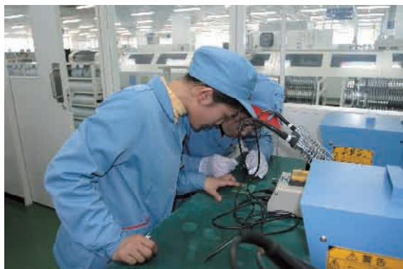
▲ MDI is working to use lead-free soldering in circuit boards. Lead-free soldering takes considerable skill. Here a skilled worker gives instructions to a junior worker.
