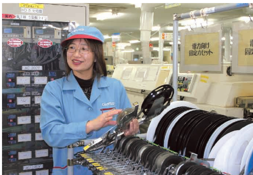
▲ "We were able to get people to think about energy intensity in terms of productivity," says Yuko Kaneshima. By introducing color-coded indicators on the fixed cassettes containing chip devices [foreground in photo] we were able to improve procedures and make them easier for anyone to identify, reducing time losses.
