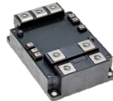
LV100-type 2.0kV IGBT Module for industrial use
